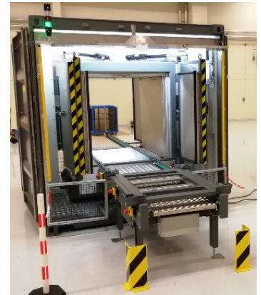
HWM-1800C in a 5-foot container incl. conveyors on the entrance and exit side (option)
